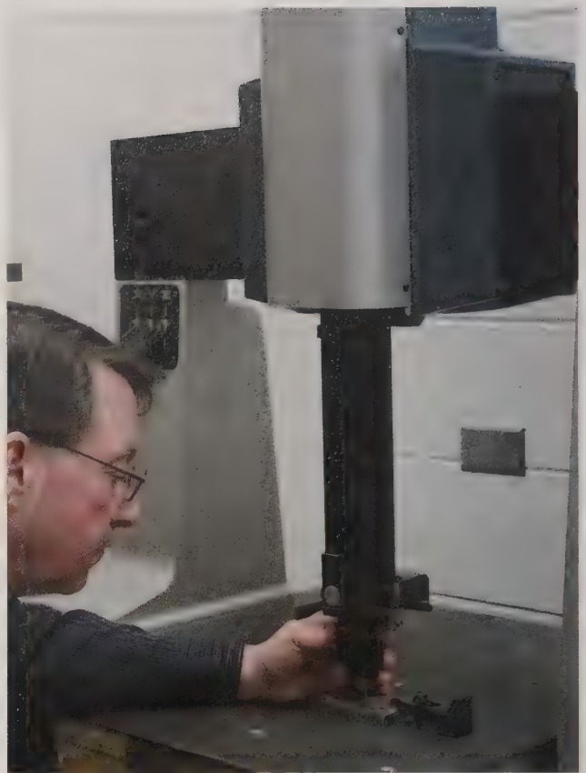
Figure A-2 Quality control technician using a CMM to inspect a part (Courtesy of Fox Valley Technical College).
