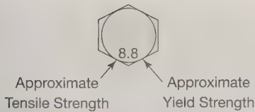
Figure A-19 Strength class marking for metric bolts (Courtesy of Fox Valley Technical College).
