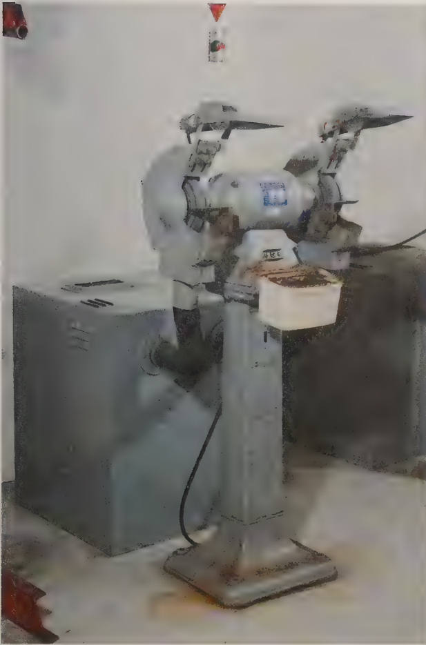
Figure A-6 Dust collector installed on a grinder.
