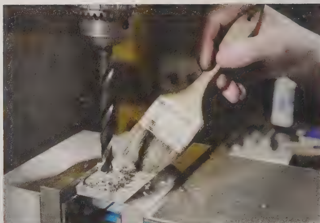
Figure A-9 Use of a brush to remove chips safely.
