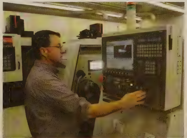
Figure A-1 Machinist programming a part on a CNC turning center (Courtesy of Fox Valley Technical College).
