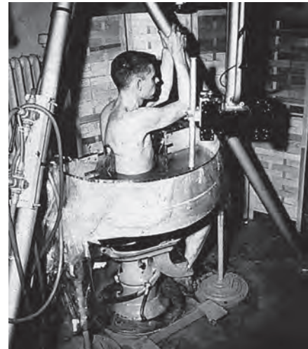
FIG. 1.3 The Pan Scanner , put together by the Holmes, Howry, Posakony, and Richard Cushman team in 1957, was a landmark invention in the history of B-mode ultrasonography. With the Pan Scanner , the patient sat on a modified dental chair strapped against a plastic window of a semicircular pan filled with saline solution while the transducer rotated through the solution in a semicircular arc.
