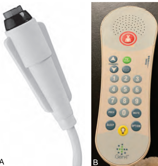
FIG. 2.2 (A) A simple call button. Pressing the button will cause an alarm to go off. This is usually the type of call bell found in an ultrasound department. (B) A call button that can also control the television in a patient's room. Pressing the red button on top with the nurse icon will notify someone that the patient needs help, causing a light to flash and an audible signal. The cancel button is typically in the patient's room, requiring a staff visit when it is pressed.
