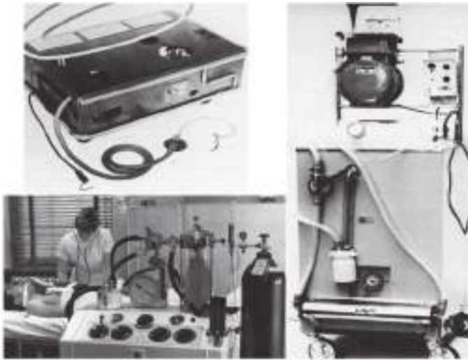
Fig. 1.8 Top left, Morch ventilator; bottom left, Engstrom 300 ventilator; right, Emerson post-op ventilator. (From Mushin WW, Rendell-Baker L, Thompson PW, Mapleson WW: Automatic ventilation of the lungs , Oxford, 1980, Blackwell Scientific.)
